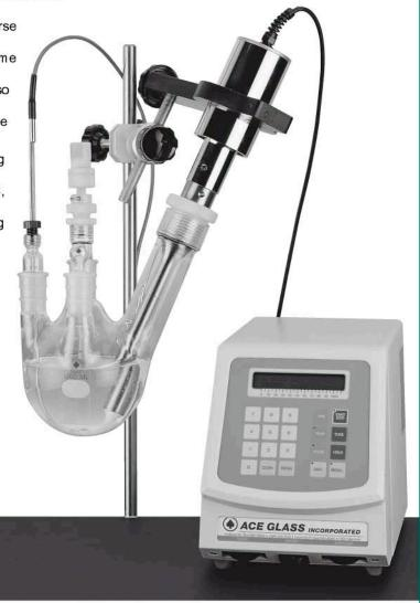
Originally, because of their availability, conventional, low power ultrasonic cleaning baths were used in the laboratory for Sonochemical investigations. Although these baths were somewhat effective with very reactive metals, the intensity was not localized and insufficient for most Sonochemical reactions. In addition, variables such as level and temperature of the liquid, position within the bath, and inconsistency of power output were numerous, rendering the results hardly quantifiable.
