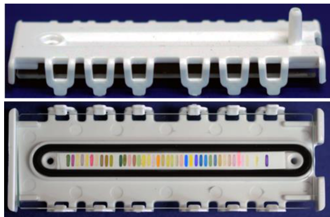
Figure 1. Photographs of the cartridge and a colorimetric sensor array showing side and array views. The sensor array shown here has 40 sensor elements at 1.2 mm center-to-center spacing and represents typical printing quality.
