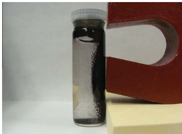
Fig. 10 – Magnetic separation of the Fe–C composite from a suspension in water.
