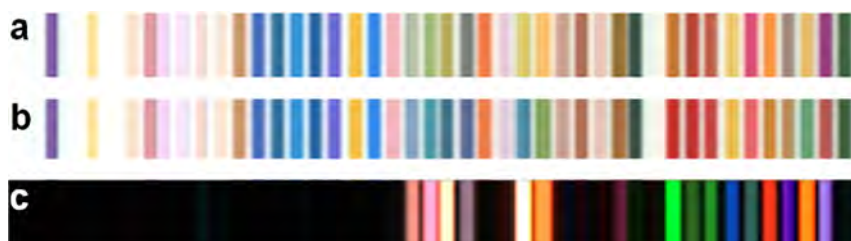
Figure 21. Digital images of the 1 \times 40 colorimetric sensor array (a) before and (b) after exposure to headspace gas of ammonium nitrate, and (c) a scaled color difference map generated from the subtraction of the before and after exposure images. The color difference map represents the difference vector in 120 dimensions. For purposes of display, the color range of difference maps is usually expanded from the effective dynamic range to the full RGB display range (i.e., 4 bit color expanded to 8 bit color scale in this case, or 0–15 expanded to 0–255 in RGB values). Reproduced with permission from ref 32. Copyright 2016 Royal Society of Chemistry.
