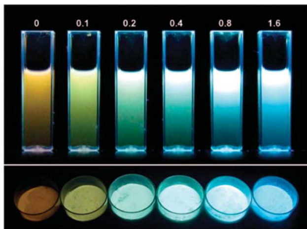
Fig. 16 Photographs (under UV light) of ethanol solutions (upper) and dry powders (lower) of Mg/ZnO nanoparticles prepared by ultrasonic irradiation of ZnO with \text{Mg}^{2+} with different Mg/Zn ratios. Reprinted with permission from ref. 60. Copyright 2009 John Wiley & Sons.
