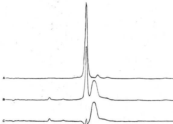
Figure 3. IR spectra from a kinetic run. Spectrum A is the initial spectrum of Mo(CO)_6 in the presence of a 10-fold excess of P(O)Ph_3 ; spectrum B is the spectrum after 55 min at 110 °C; spectrum C is the optimal difference spectrum showing only the contributions of Mo(CO)_5(P(O)Ph)_3 . The spectral range is from 2200 to 1750 cm^{-1} .
