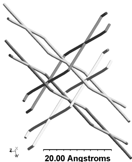
Fig. 3. Schematic of porphyrin bands showing interpenetration of orthogonal bands. Outside vertices of the diamond correspond to location of the calcium ions within solid-state packing model; crossing of cylinders corresponds to the center of the porphyrin macrocyclic plane. The primary building unit of the extended solid-state structure, the bands interpenetrate at half-porphyrin unit intervals in both directions
