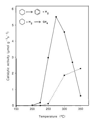
FIG. 4 The catalytic activity of amorphous and crystalline iron powder as a function of temperature for the cyclohexane dehydrogenation and hydrogenolysis reactron. Solid line, amorphous iron powder, prepared sonochemitally from Fe(CO)<sub>5</sub>; dashed line, crystalline iron powder (5-km dtameter. Aldrich Chemicals).
