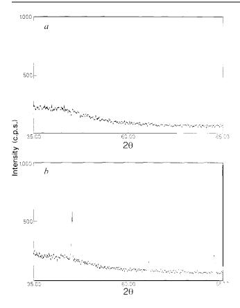
FIG. 3 X-ray diffractron powder patterns of amorphous iron powder (a) before heat treatment and (b) after crystallization at 350 °C for 6 h. Data collected on a Rigaku D-max diffractometer.
