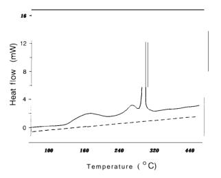
FIG. 2 Differential scanning calorimetry of amorphous (solid line) and crystalline (dashed line) iron powders, obtained at 10 °C min<sup>-1</sup> on a DuPont 1090 calorimeter
