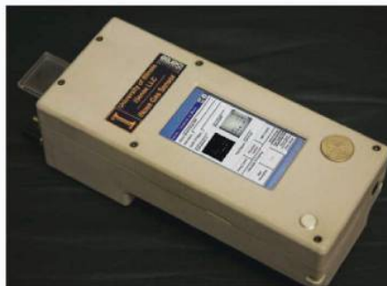
The handheld device that houses the array of chemical-detecting pigments is about the size of a deck of cards.
