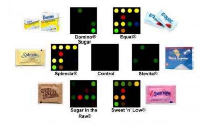
In an advance toward a long-awaited "electronic tongue," a new sensor can detect up to 14 common used sweeteners. The device shows promise for quality control monitoring in the food and beverage industry. (Image: Kenneth Suslick, Ph.D., University of Illinois at Urbana-Champaign)
