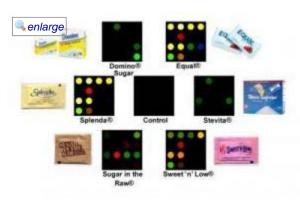
In an advance toward a long-awaited "electronic tongue," a new sensor can detect up to 14 commonly-used sweeteners. The device shows promise for quality control monitoring in the food and beverage industry. (Credit: Kenneth Suslick, Ph.D., University of Illinois at Urbana-Champaign)
