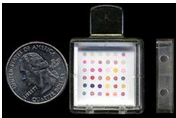
SPOT ON. The dabs of dye on this coin-size sensor change color in response to odors.
